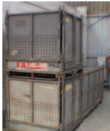
The parts are removed and put away securely out of the way, eliminating damage to fittings and reducing the H&S risk.
